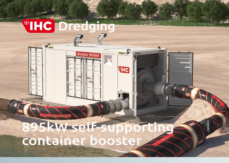
The Royal IHC 895kW booster is a versatile and robust booster station that is equipped with state-of-the art technology and significantly improves the productivity of your dredger over longer pumping distances. The option to adapt to pipelines ranging from 400 to 500mm enables your vessel to work across various dredging projects. The pump system is reliable, fuel-efficient and has low maintenance costs.
