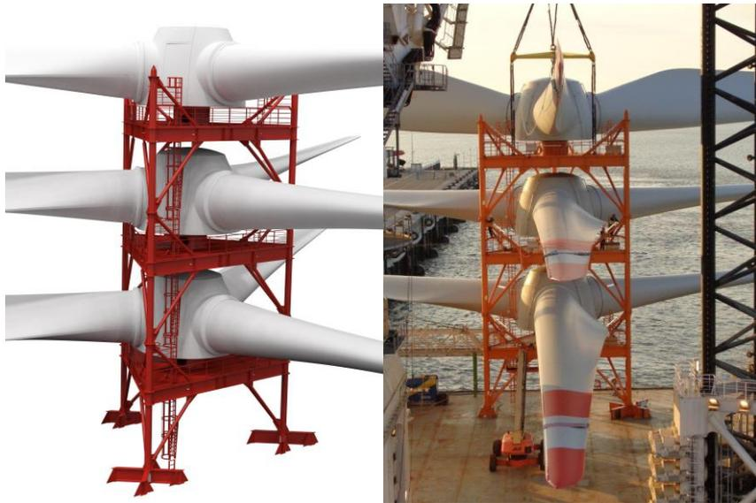
Taking a closer look into seafastenings on self-elevating platforms it can be seen that a weight reduction can lead to a significant operational advantage. Lighter seafastening will require less deck space resulting in more room for paid cargo. Subsequently the jack-up vessel can transport more payload. In case the weight savings are translated to additional consumables, a higher autonomy can be obtained resulting in fewer round trips.
