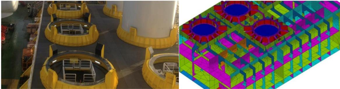
Above pictures shows the optimized grillage design in finite element modelling (FEM).
