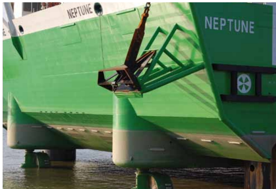
In the bow, the pods' lower gearboxes are housed in gondolas
