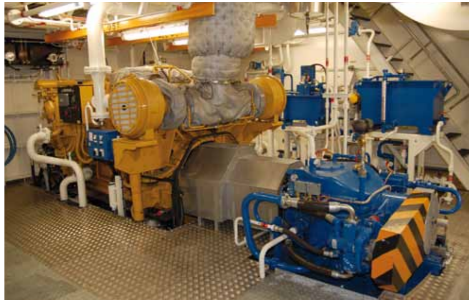
Four completely independent engines/pod units provide the propulsion and steering
