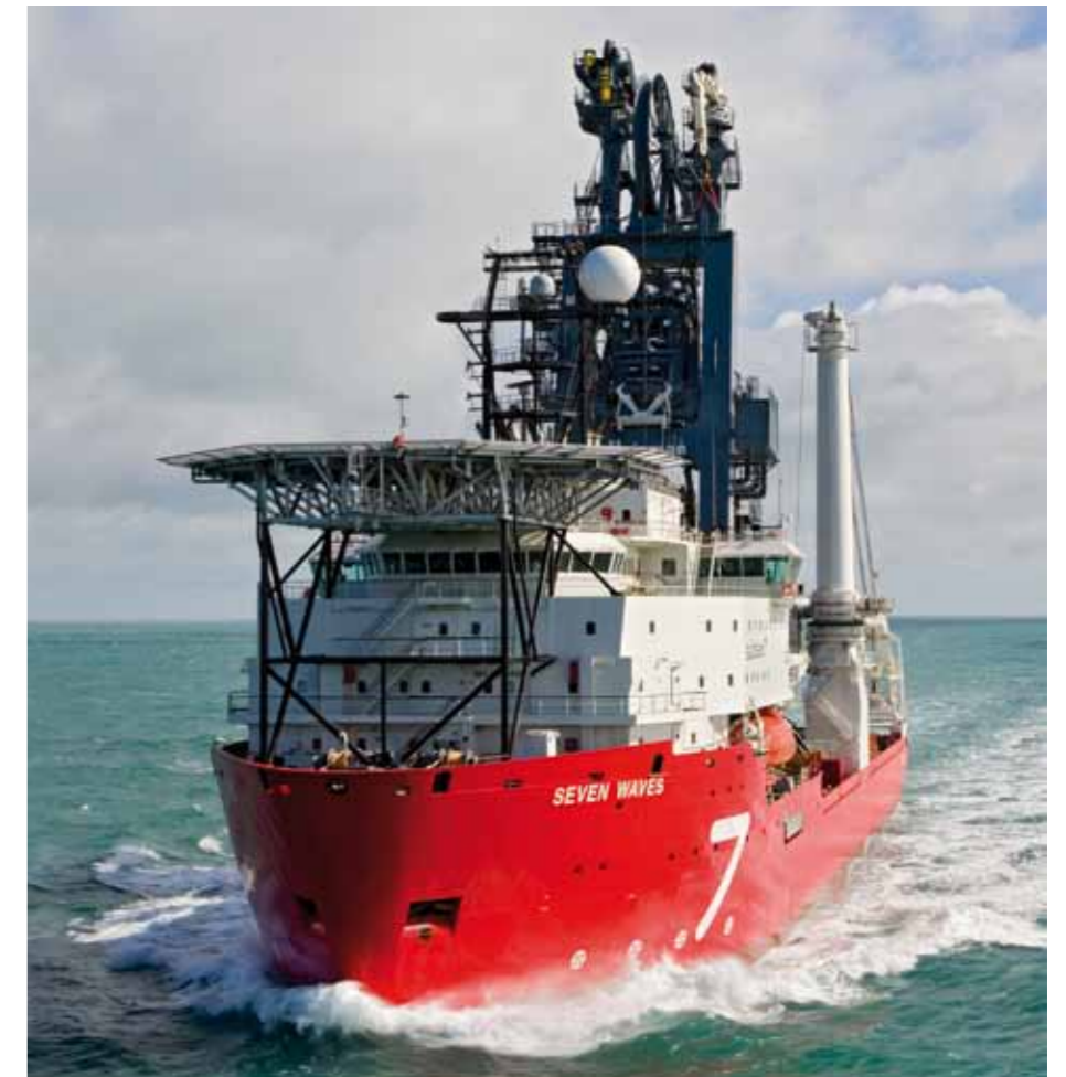
The helicopter deck, on deck ten forward of the superstructure, is an approved and certified platform
