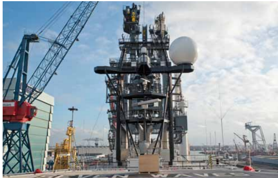
The largest TLS ever produced at Huisman, seen from Helicopter deck, behind the mast with communication equipment
