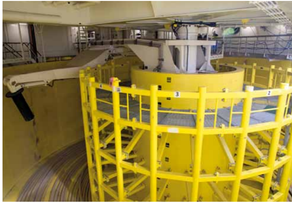
The core diameter of the carousels can be increased by means of placing a so called 'false core' (a cage like structure)
