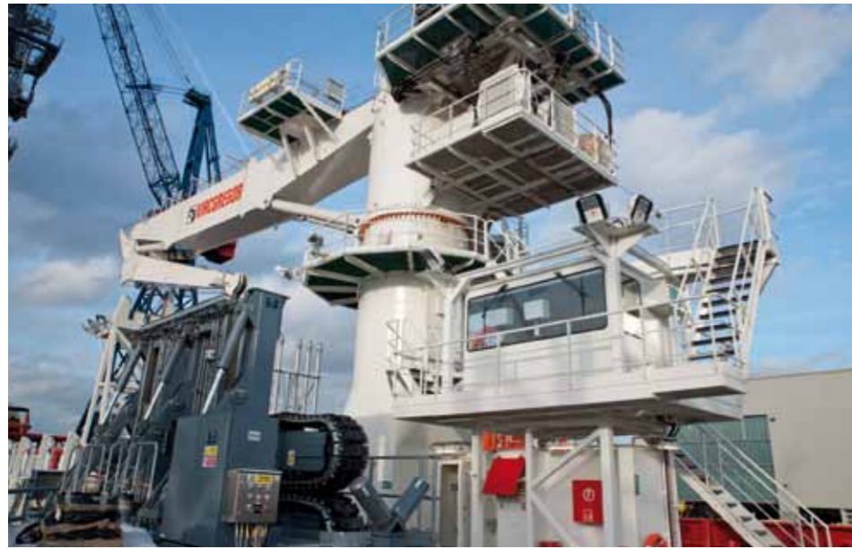
The second largest crane on board is a knuckle boom, which is on starboard side behind the carousels
