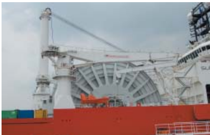
The 3500 ton capacity main reel is located in a well on the main deck
