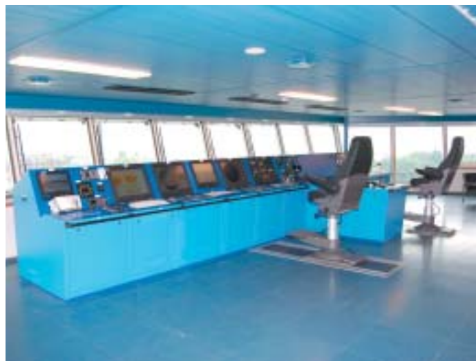
The navigation bridge is one of four control stations in the wheelhouse
