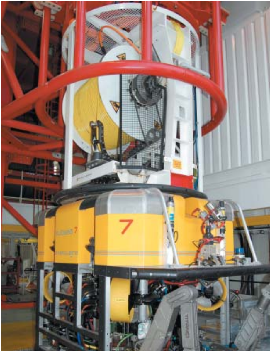
The ROV's are launched in a protective cage
