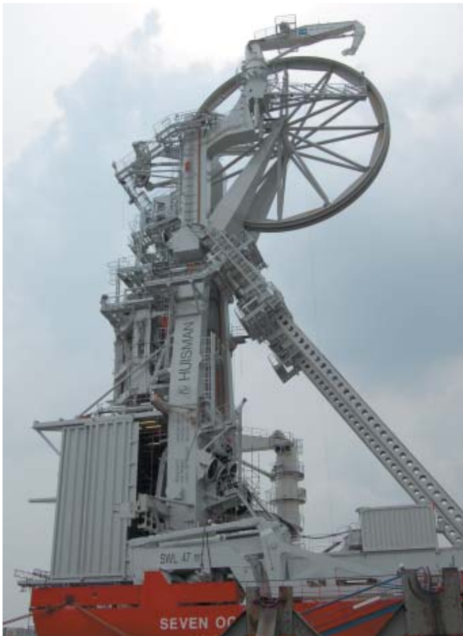
The lay ramp is placed on a skid beam and can be tilted forward
