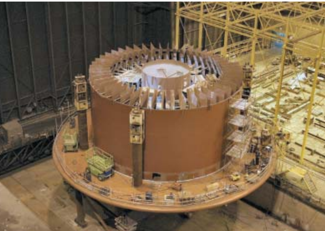
* The main reel has a diameter of 28 metres and is 10 metres wide
