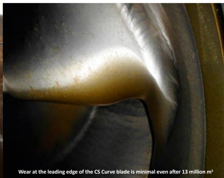
Wear at the leading edge of the CS Curve blade is minimal even after 13 million m<sup>3</sup>
