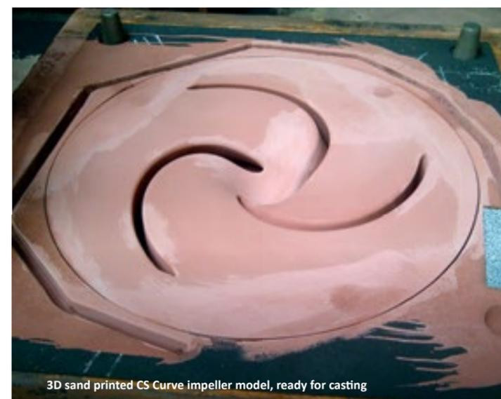
3D sand printed CS Curve impeller model, ready for casting
