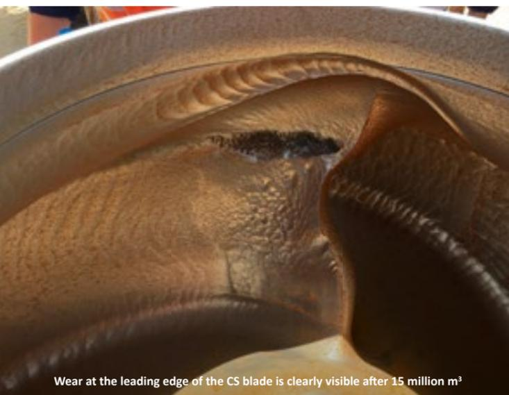
Wear at the leading edge of the CS blade is clearly visible after 15 million m<sup>3</sup>
