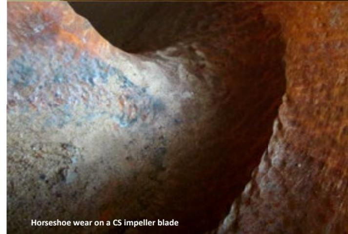
Horseshoe wear on a CS impeller blade
