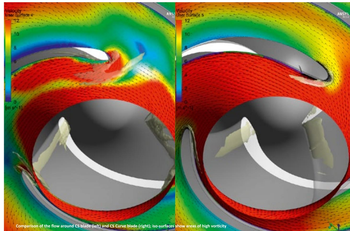
Comparison of the flow around CS blade (left) and CS Curve blade (right); iso-surfaces show areas of high vorticity
