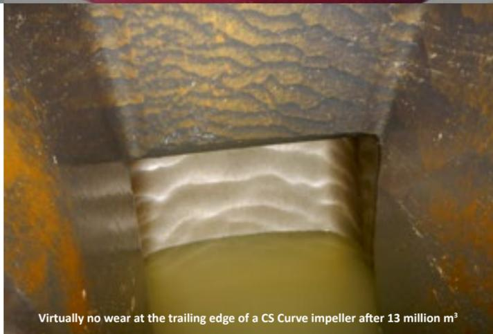
Virtually no wear at the trailing edge of a CS Curve impeller after 13 million m<sup>3</sup>
