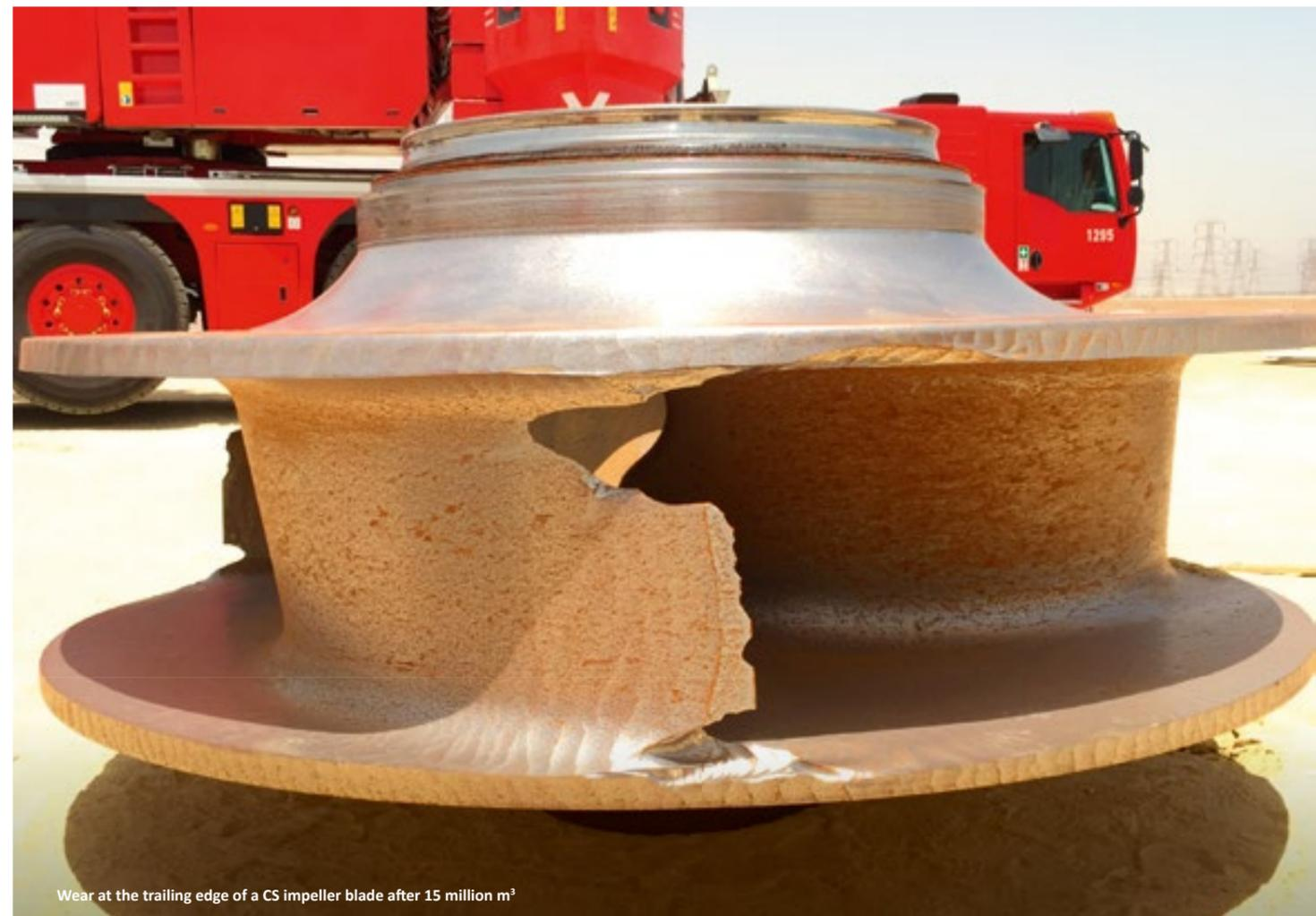
Wear at the trailing edge of a CS impeller blade after 15 million m<sup>3</sup>
