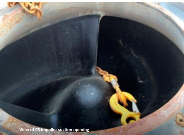
View of CS impeller suction opening
