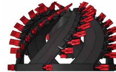
CUTTER HEAD WITH TEETH CONNECTED TO WING ADAPTER
