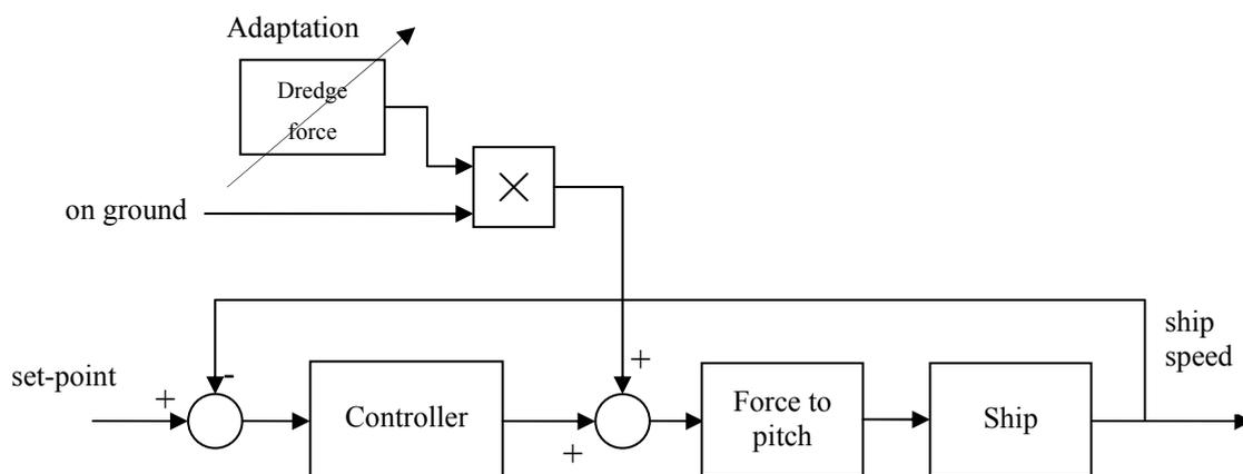
Figure 5. Schematic overview of the Trail Speed Controller.
