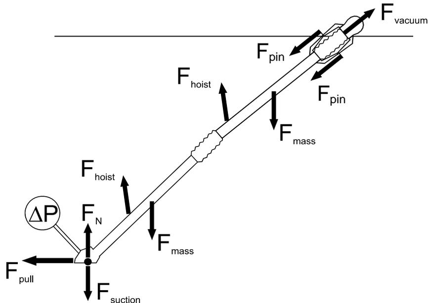
Figure 3. Forces acting on suction tube.
