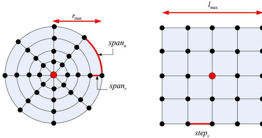
Figure 12. A circular and square grid of points for the approximated minimum search.
