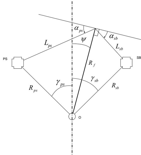
Figure 11. Reference system Anchor position estimator.
