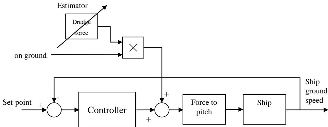
Figure 4. Schematic overview of the Trail Speed Controller.
