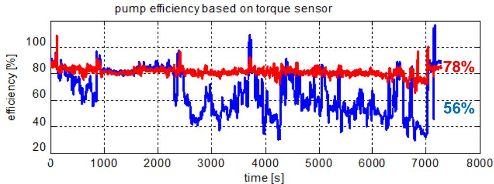
Figure 7. Efficiency of cavitating pump (blue) versus non-cavitating pump (red)
