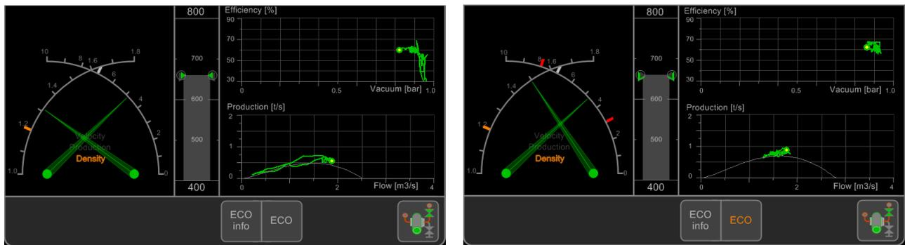
Figure 11. Dredging process with controllers enabled (right) and disabled (left)
