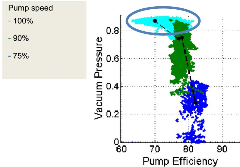
Figure 6. Reduced pump efficiency.
