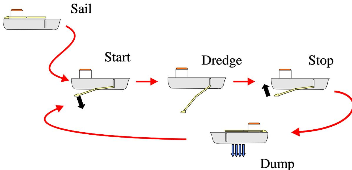
Figure 1. Dredging cycle of a hopperdredge.
