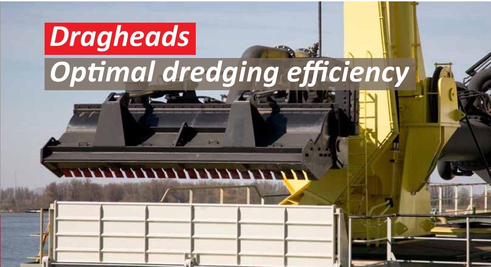
The draghead on a trailing suction hopper dredger is the first mechanical point of contact with the materials at the bottom. Its design, quality and sturdiness are critical to the dredging process. IHC Parts & Services has invested many years of practical experience and testing to create optimal draghead solutions, which are capable of extracting the maximum amount of soil from the bottom within the shortest possible time and at minimal cost.
