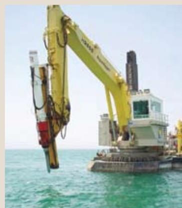
Demag with IHC Hydrohammer® rock breaker
