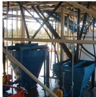
**SLURRY PROCESS BINS FOR SAND TRANSFER DUTIES**
