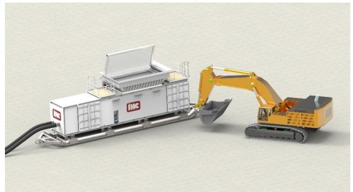
Using slurry pipeline transport instead of a large truck fleet, increases operational safety and reduces the costs per tonne. And with the completely electrified slurrification unit, also adds to a low carbon foot print significantly.
