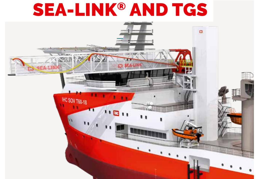
The Sea-Link® provides a safe and rapid transfer between a vessel and an offshore structure. Personnel are able to cross the Sea-Link® at any time via a direct connection, which guarantees a time-efficient operation. Utilities (electrical power, grout, water and fuel) and cargo can also be transported safely over the Sea-Link®. The system incorporates active motion compensation of the tip allowing it to stabilise respond to any of the vessel's six degrees of freedom (6DoF).
