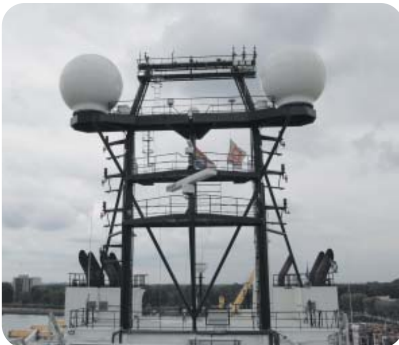
The mast houses two radars and two large satellite domes for communication
