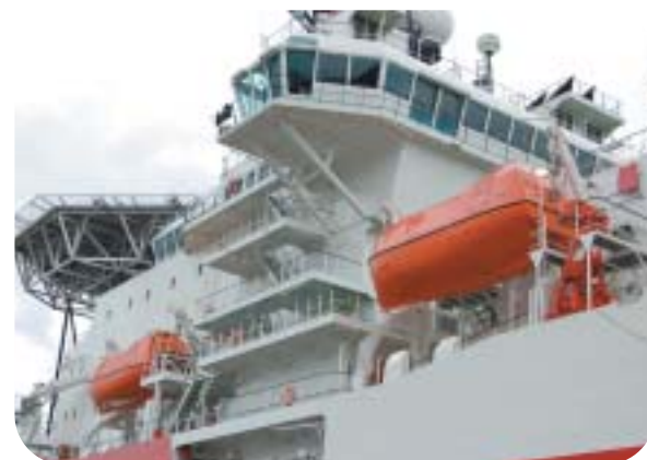
Two hyperbaric lifeboats can evacuate divers while maintaining pressure conditions
