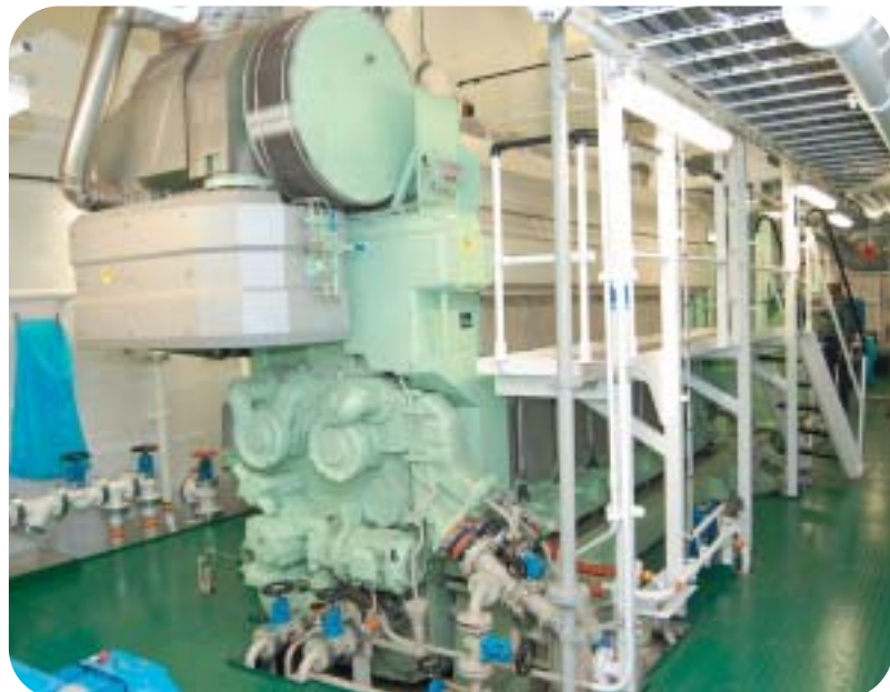
Power is generated in six diesel generators divided over three engine rooms
