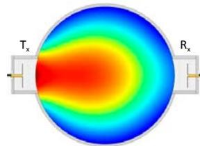
The measurement is done by a pair of antennas fitted to the slurry pipeline. The transmitting antenna ( $T_x$ ) creates an electromagnetic field, which penetrates the mixture in the pipe. Field is sensed by the receiving antenna ( $R_x$ ). Solids present in the carrier fluid affect the received signal amplitude and phase. Those parameters are measured by an electronic circuit, and used for calculation of the concentration.
