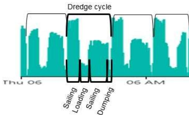
Figure 2: Expected speed over time track of a Trailing Suction Hopper Dredger
