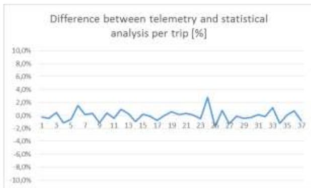
Figure 5: Difference per dredging trip between the statistical analysis and the vessels telemetry.
