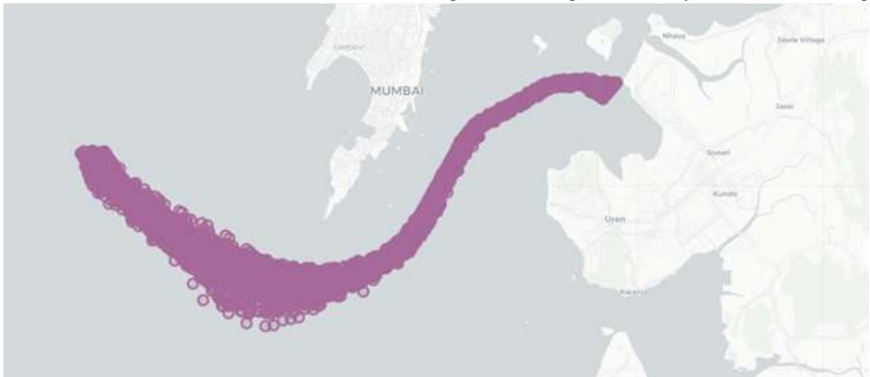
Figure 3: Operational activity of an 8,000m<sup>3</sup> TSHD in the port of Mumbai in January 2019
