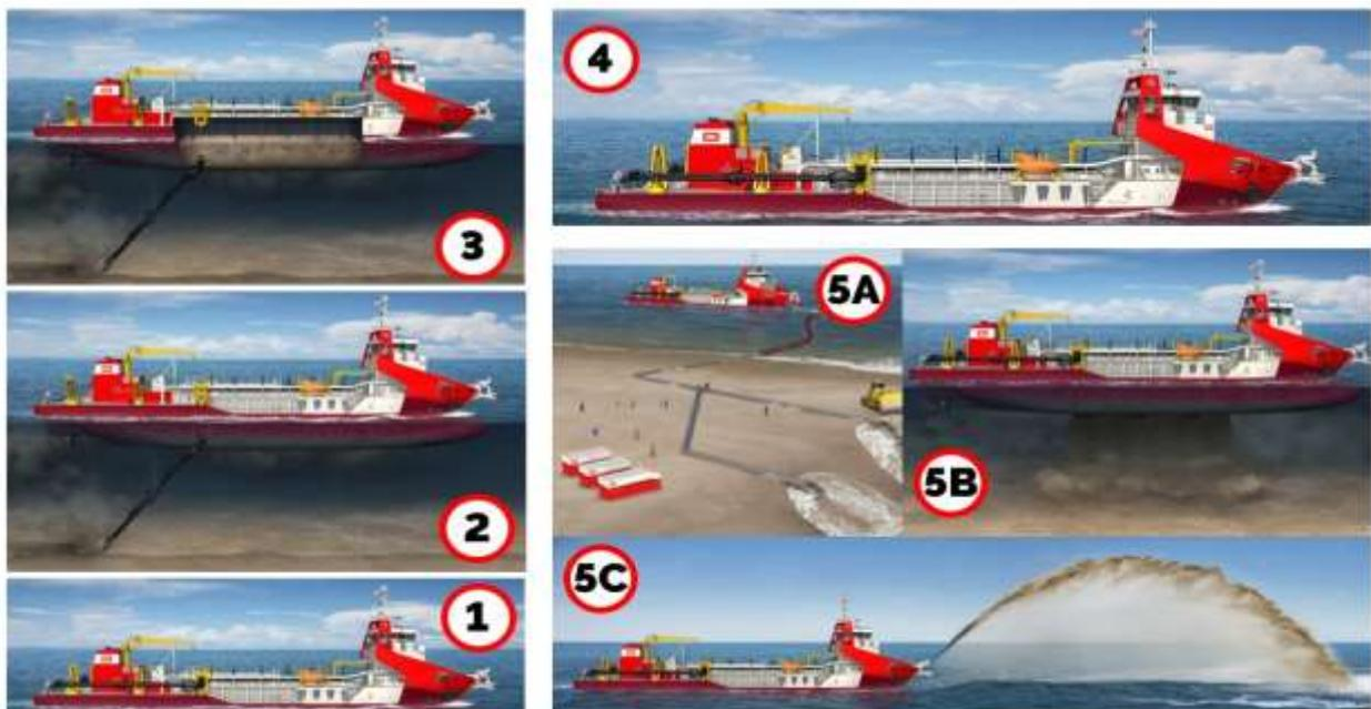
Figure 1: Graphical representation of a dredge cycle
