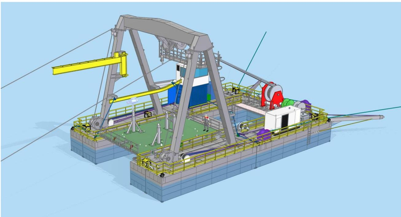
*Arctic Canadian Diamond Company and IHC Mining's Launch and Recovery Platform for the Underwater Remote Mining System, which will help recover diamond-bearing kimberlite ore from deep open pits at the Ekati Diamond Mine in the Northwest Territories of Canada.*
