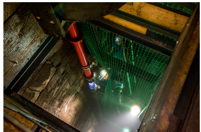
FIG. 12. THE VERTICAL TRANSPORT TESTS AS CONDUCTED IN HALSBRÜCKE, NEAR FREIBERG, GERMANY, ARE TRULY UNIQUE IN SIZE AND SCOPE. THE 136 M LONG TEST SECTION BELOW SURFACE LEVEL (TOP), SURFACE LEVEL SEDIMENTS PLANT AND PUMP STATION (MIDDLE) AND A LOOK DOWN THE MINESHAFT (BOTTOM).
