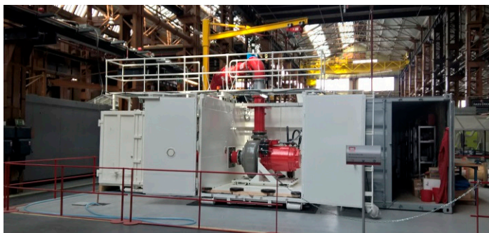
FIG. 8. MEMBER TYPE CONCEPT BOOSTER STATION FOR THE VTS, CONSISTING OF TWO CENTRIFUGAL DREDGE PUMPS AND SEVERAL VALVES.
