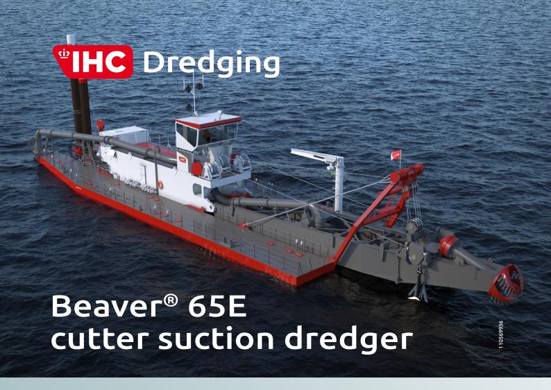
The Beaver® 65E is a fully electrically powered version of the standard Beaver®. With zero emissions and limited noise disturbance, the Beaver® E fully complies with the latest environmental regulations and is therefore also suitable to work in the most sensitive environments.
