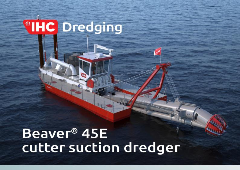
The Beaver® 45E is a fully electrically powered version of the standard Beaver®. With zero emissions and limited noise disturbance, the Beaver® E fully complies with the latest environmental regulations and is therefore also suitable to work in the most sensitive environments.
