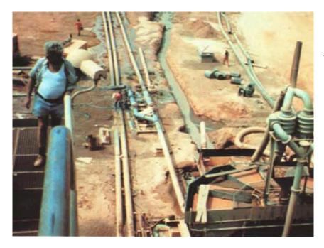
The primary stage concentrate is fed into the secondary jig stage, of which the tailings are recirculated via the primary stage. The secondary stage concentrate is further upgraded in the tertiary jig stage, producing the final con-centrate. Tailings from the tertiary stage are also recirculated via the secondary stage.
