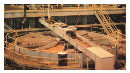
This results in a higher percentage of gold than average material recirculating in the ballmill circuit. and is known as overmilling of the gold. The installation of a gravity step will reduce this effect, as the gold will be recovered before it can be recirculated by the cyclone. Moreover, gold particles with an oxidized coating will be concentrated by the gravity step, whereas certain chemical processes will have problems.
