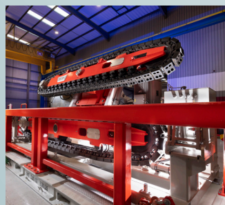
◀ 15-tonne breakback tensioner with bi-directional cable passing, available to rent from Royal IHC
