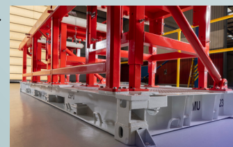
◀ 15-tonne breakback tensioner with bi-directional cable passing, available to rent from Royal IHC
