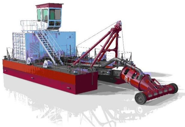
OTTer® 250 dredger with auger and ladder in upward position
