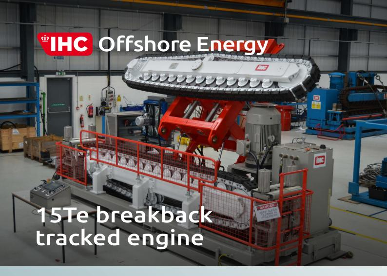
Our 15Te tracked engines, Rigs 113 and 114, are designed to be used in the laying and retrieval of subsea cables used within such industries as the power industry and telecommunication industry.
