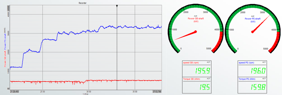
Measurement data showing the maximum power on the PS propulsion shaft
